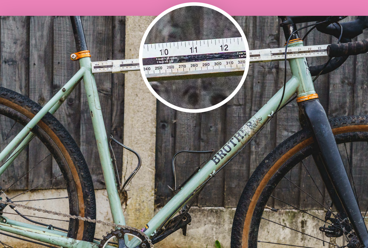
Figure 1. Tape a ruler to the top tube of your bike.
